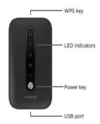
**Power key**: Hold the Power key for 3 seconds to power the device on/off. When the screen is off, press the Power key to turn the screen on.
